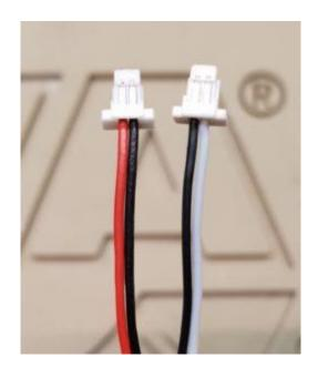
Black is not always negative! The wires that may come with your unit and go from the switch to the hop could be coloured black and white. In this instance....
