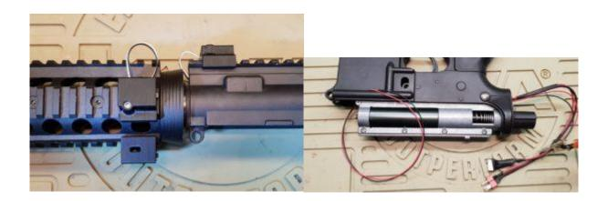
Also considerer the route for the power supply wires. These wires have been left long, don't be tempted to cut them too short until you have at least test assembled it all together.
