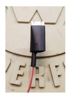
Place the larger piece of shrink wrap over the connector, if necessary you can stretch the shrink-wrap to make fitting easier.
