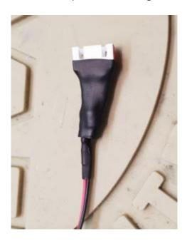
When this is heated the glue will melt inside and make the whole thing well protected and solid.
