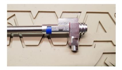
Now is a good time to check that the feed lips don't look distorted. Put a bb in the hop unit and using a cleaning rod or similar push the bb through the hop lips, it should pass easily with little resistance. If it is hard to push through then the bucking could have stretched or distorted whilst fitting, or your barrel/bucking/hop unit may have compatibility problems. If you have a problem then it needs to be fixed before moving on to the next step.
