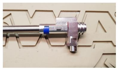
Visually check how the window in the barrel lines up with the window in the hop unit, you can increase the size of the barrel window if required.
